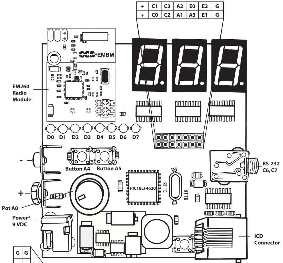
\*Use only one power source, either wall adapter or battery.
