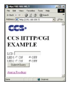
The website uses an HTML input form to change the data displayed on the LCD and to change the status of the two LEDs. Click on the "Analog Readings" link to go to another page on the prototyping board server that displays the current ADC readings of AN0 and AN1.
