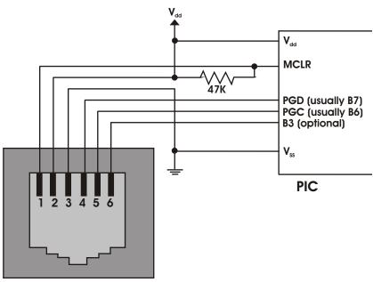
Target ICD connector Looking into the connector
