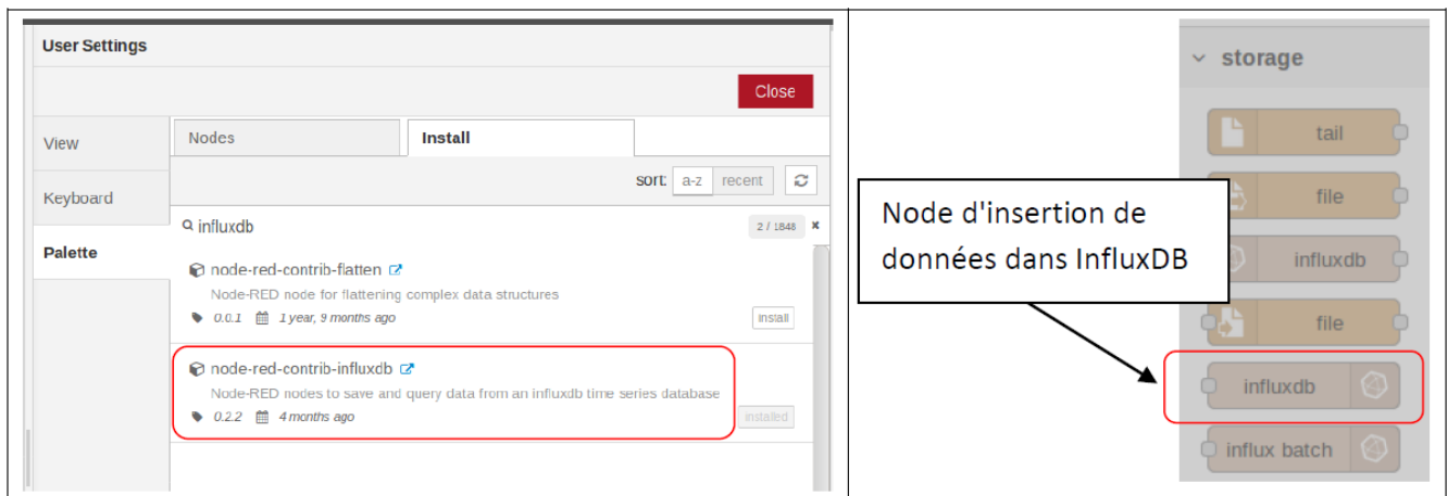
Figure 31. Installation des nodes node-red-contrib-influxdb
